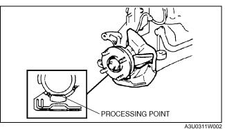
3. Tighten the hub nut while holding the wheel hub using a brass bar.
